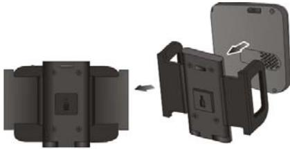
1. Insert the device into the car holder.
